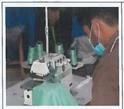
1- Over lock machine has no eye guard (Safety and Hygienic Conditions-3, NC No-1)
